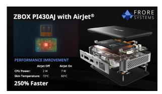
Zotac Mini PC - achieving a 250% increase in performance: The world's first Mini PC with AirJet, the Zotac ZBOX PI430AJ PICO with AirJet® increases sustained CPU performance by 250% while lowering skin temperature by 12°C, making it the smallest, most powerful Mini PC available.
